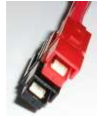
Figure 3: PowerPoles joined "red over black." Note the hood and peg positions.
