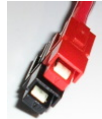
Figure 3: PowerPoles joined "red over black." Note the hood and peg positions.
